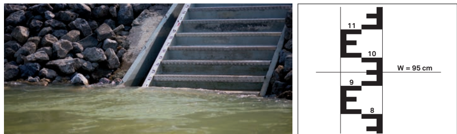
Gauge staff at a gauging site; sample water level at gauge: 95 cm
