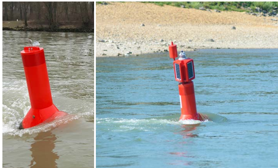
Use of remote monitoring technologies on plastic buoys of the type B7 (without light) and LT B7 (with light); on the left: monitoring using Globalstar (satellite); on the right: monitoring using AIS
