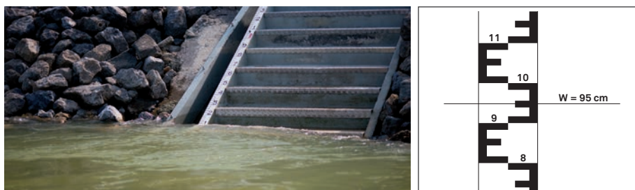
Gauge staff at a gauging site; sample water level at gauge: 95 cm
