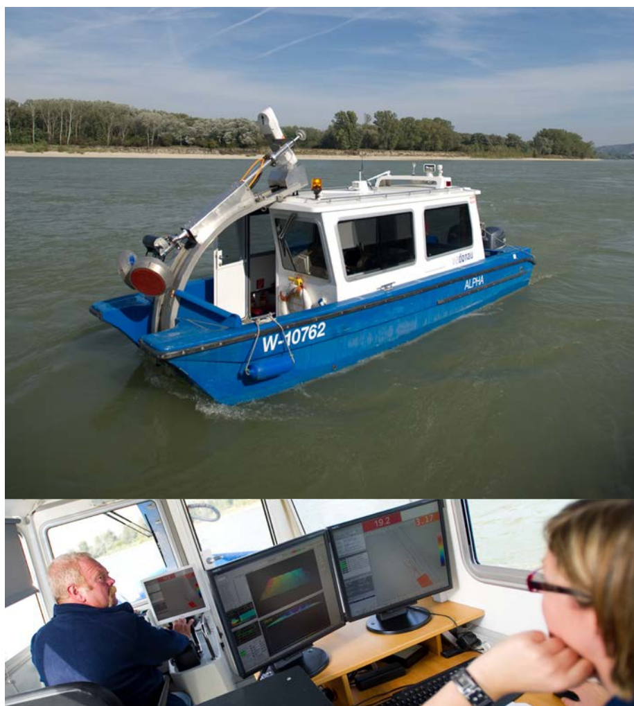
Multi-beam bathymetric survey on the free-flowing section of the Danube east of Vienna by via donau – Österreichische Wasserstraßen-Gesellschaft mbH
