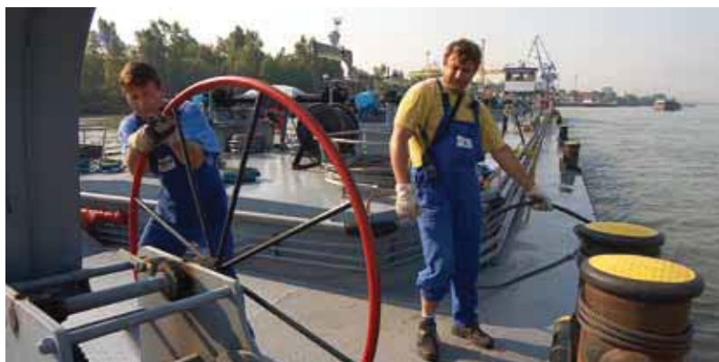
Crewmen connecting a tank lighter
