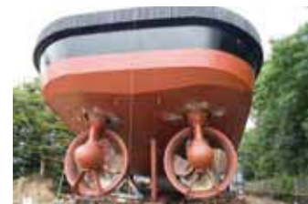
Twin-screw propulsion with ducted propellers
