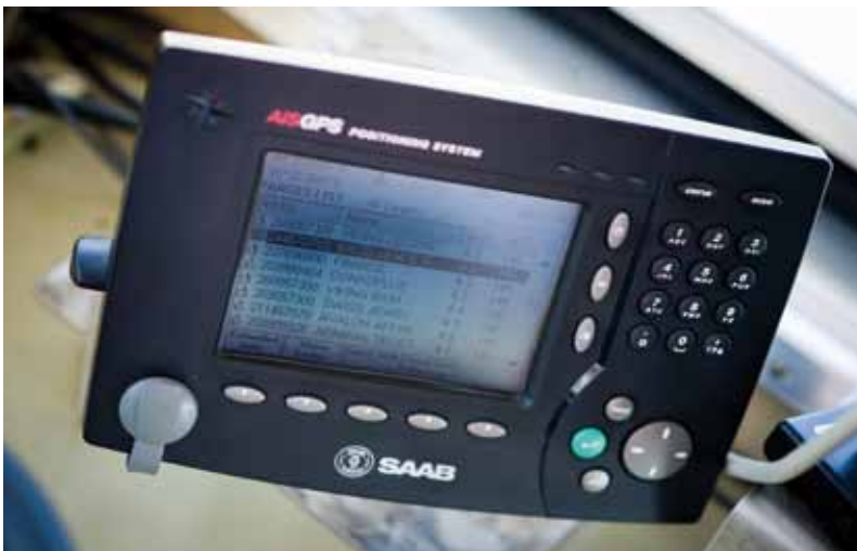
AIS transponder on board an inland vessel
