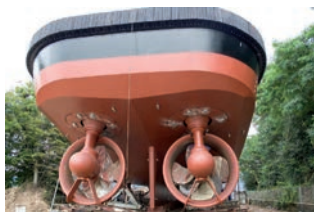
Twin-screw propulsion with ducted propellers
